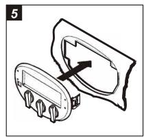
Make all wiring connections to the Integrated Mounting Kit and snap the assembly into the sub-dash. Reach under the driver's side dash and re-attach the temperature control cable.
